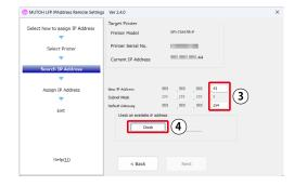
2. Enter a new IP address directly (③). Click [Check] (④) to check if the IP Address entered can be assigned for the machine.
