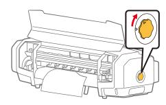
Pull out the media and cut the torn area with a cutter.
