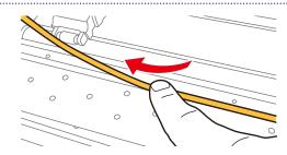
Attach the edge holders from the left side of the platen.
