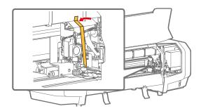
Secure the sheet cutter with tape.
