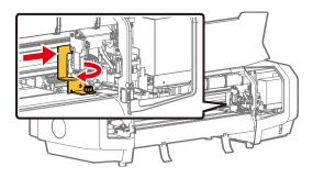
Secure the contour cutter with tape.
