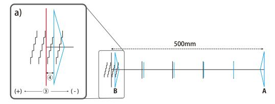
Example b) If the width of the pattern is set to 500 mm and the cut line was off from the reference line by eight vertical lines of the scale lines to the non-origin side:
