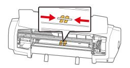
Attach the steel veyor protector and secure with tape.
