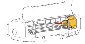
Manually move the carriage to the platen where you can easily install the blade holder.
