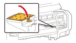
Attach a new pad to the flushing box.
