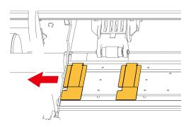
3 Slowly peel off the cutting mat to remove it from the platen.
